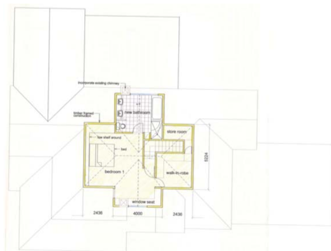
Figure 9.0, First Floor Plan, Wayne McPhee and Associates Pty Ltd in 1997 for Frances and Sean Foster. Note the one surviving chimney shown on roof plan.
